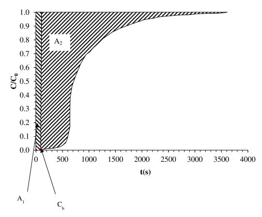
As it can be seen in this figure, we can determine the break – through time by calculating the areas  $A_1$  and  $A_2$ . Thus,
