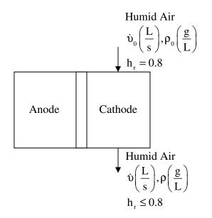
Perform a differential balance on the fuel cell for the membrane humidification process.
