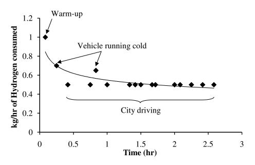
By using differential balances on the tank, determine the amount of fuel remaining in the tank after running the vehicle for 6 hours, assuming that the fuel tank is initially at its maximum capacity of 5 kg of hydrogen.
