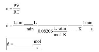
We can then use the molecular weight to determine the mass flow rate as:
